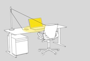
Visual task at the workstation A lighting level of 500lx is normal for office workstations, with the individual visual task not being taken into account. In many cases illuminated screens determine our everyday work. Horizontal lighting of 300lx is sufficient in such situations and this should be adaptable via a task light depending on ancillary activities and the
