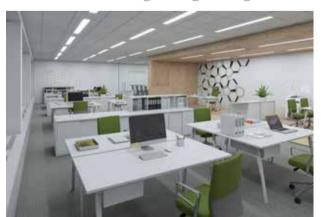
A matrix solution with panel lights does not take into account the visual task of the user. Energy needs for sufficient lighting also increase and the low-contrast impression in the space appears undefined and uninteresting.
